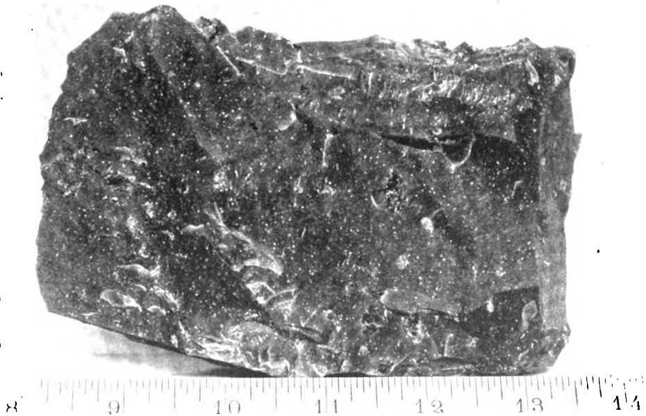
B. HANDSPECIMEN OF A VERY DENSE AND HIGHLY SILICEOUS ROCK, CONTAINING ABUNDANT AREAS OF GALENA, CHALCOPYRITE AND PYRITE. THE SMALL WHITE SPECKS ARE MINUTE AGGREGATES OF GRANULAR KAOLIN. THE ROCK IS EITHER A SILICIFIED TUFF OR DEVITRIFIED RHYOLITE. FROM ONE MILE NORTHWEST OF THE EMMONS MINE, DAVIDSON COUNTY, N. C.
